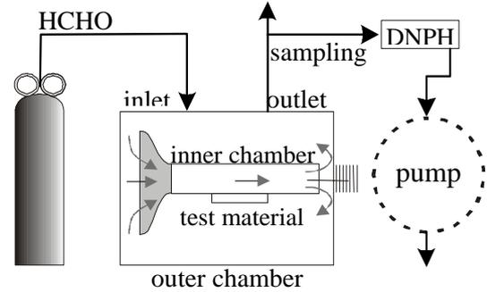
**Figure 1.** Boundary Layer Type Small Test Chamber **Figure 2.** Measurement System
