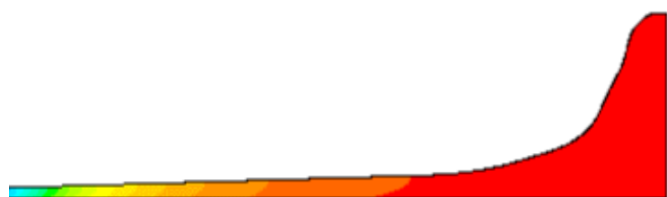
Figure 20 VOCs distribution in FLEC cavity (case of compound building materials)
