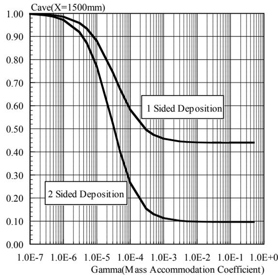
Figure 4 Average concentrations at the outlet of the test section ( $C_{ave}$ ) for various  $\gamma$  values
