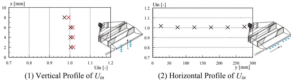
Figure 2 Flow field at supply inlet
