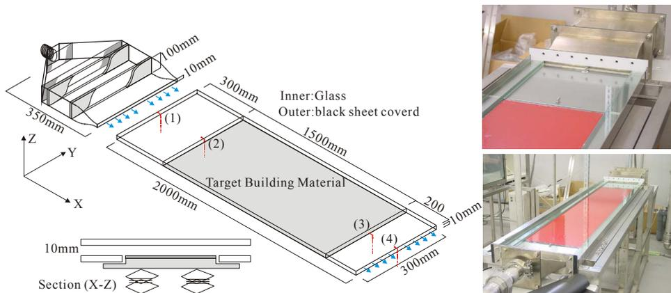
Figure 1 Perspective layout and photo of FPT Chamber
