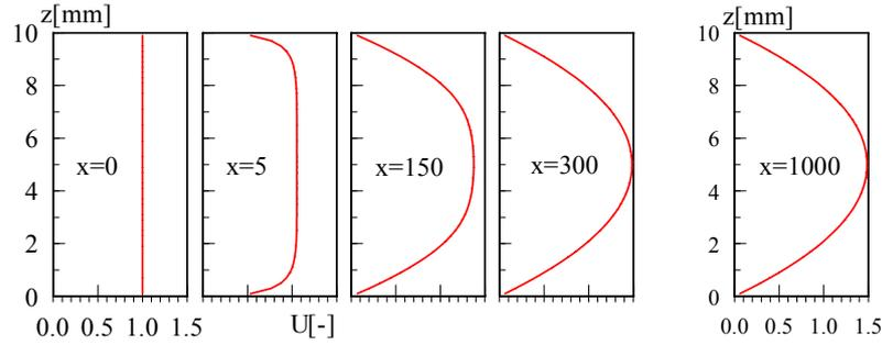
Figure 3 Vertical flow patterns along the  $x$  direction (downstream direction)
