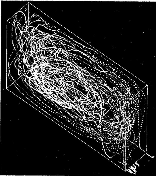
Fig. 9 Movement of eight particles from generation to exhaust
