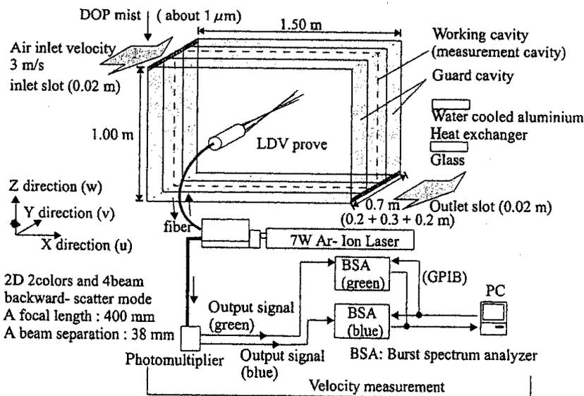
Fig. 4 Experiment model and LDV system
