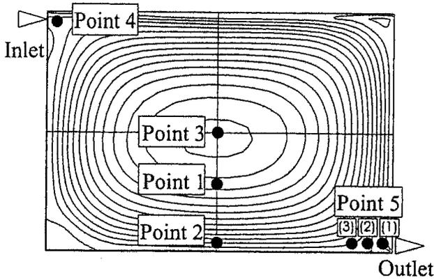
Fig. 2 Mean streamlines and particle generating points
