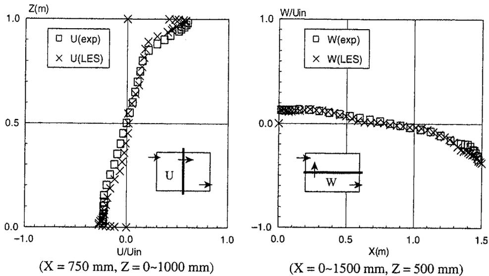
Fig. 8 Comparison between LES and experiment
