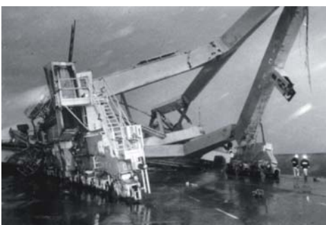
Figure 3c. Devastation of a container crane
